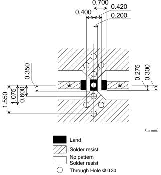
$^{\star}$  Line width to be designed to match 50 ohm characteristic impedance, Depending on PCB material and thickness.
