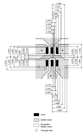
\*Line width to be designed to match  $50\Omega$  characteristic impedance, depending on PCB material and thickness.
