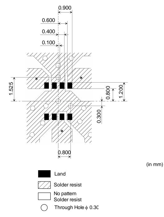
\*Line width to be designed to match  $50\Omega$  characteristic impedance, depending on PCB material and thickness.
