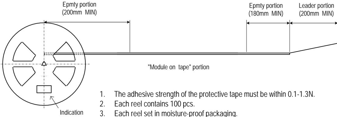
1. The adhesive strength of the protective tape must be within 0.1-1.3N.
