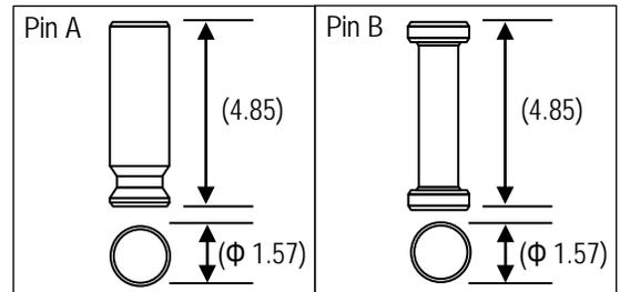
\*Pin would be used either Pin A or Pin B.
