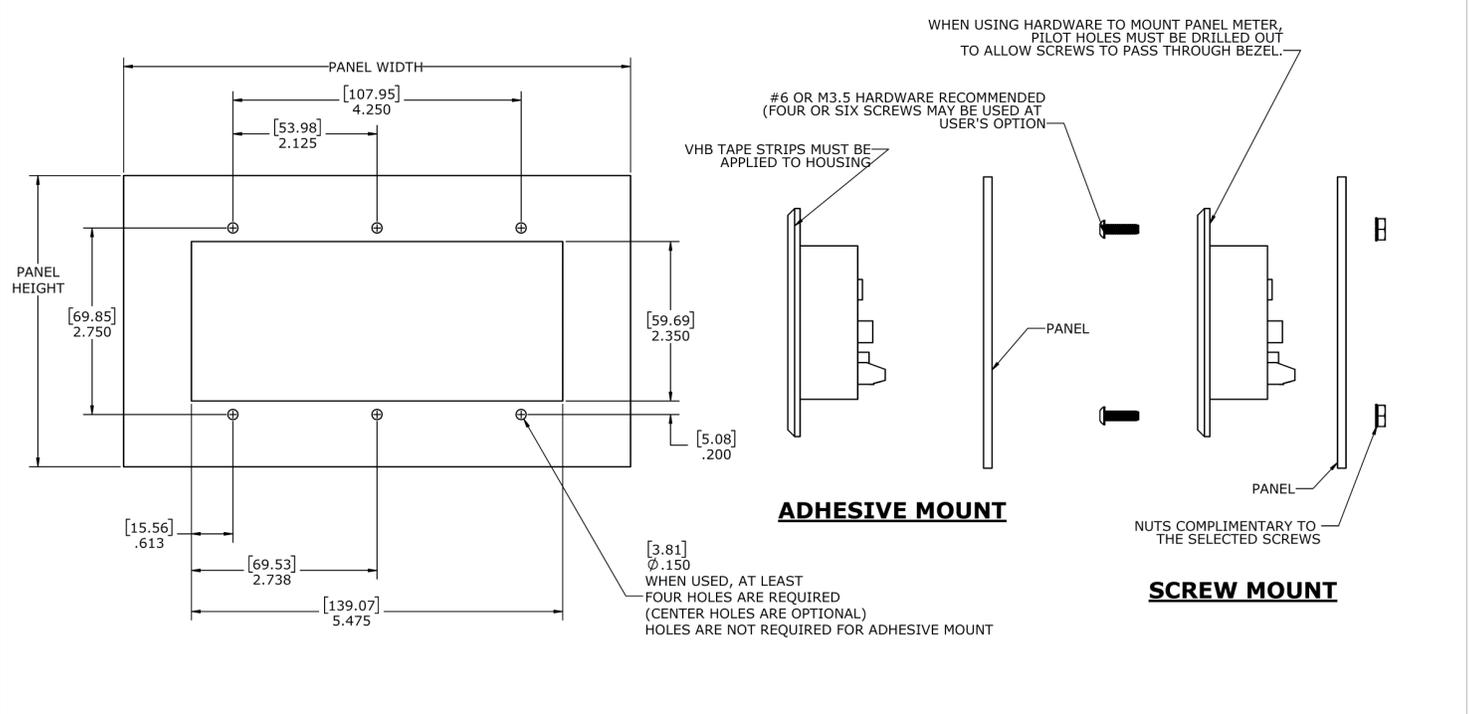
Note: When mounting panel meter with hardware, a four hole pattern (four outermost holes) or the six hole pattern may be used at the customer's option.
