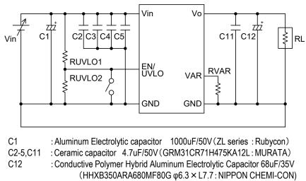
If there is a long inductive cable length between the input power source and converter, then some additional bulk decoupling capacitance (eg. up to 1000uF) may be necessary to ensure a low AC impedance power source.
