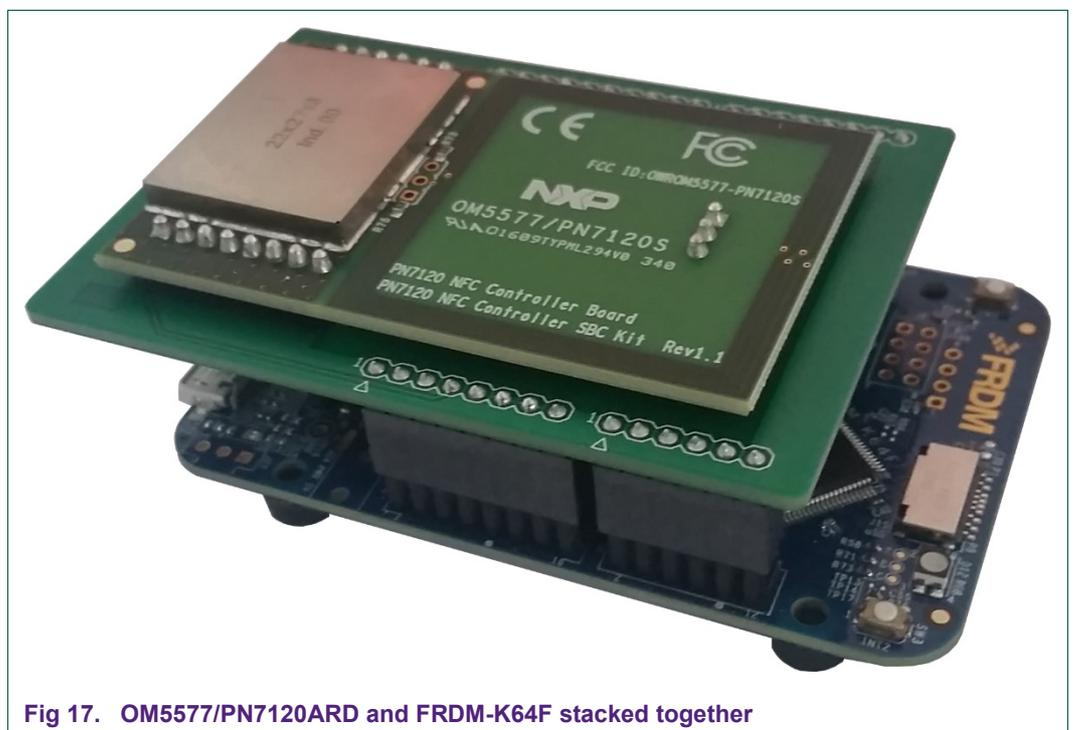
Fig 17. OM5577/PN7120ARD and FRDM-K64F stacked together
