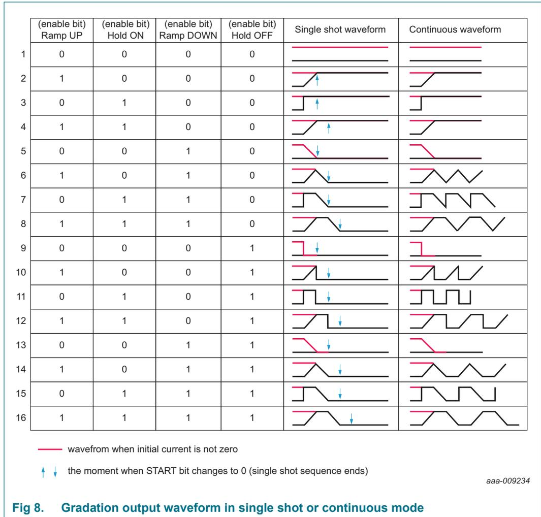
**Fig 8. Gradation output waveform in single shot or continuous mode**
