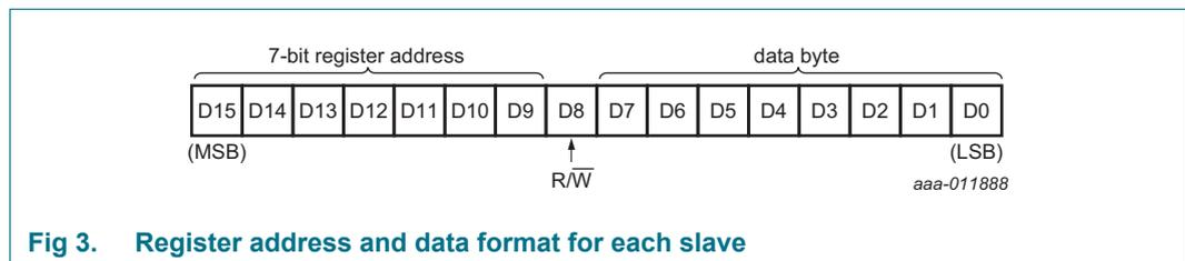
**Fig 3. Register address and data format for each slave**
