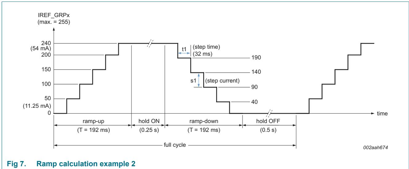
Fig 7. Ramp calculation example 2
