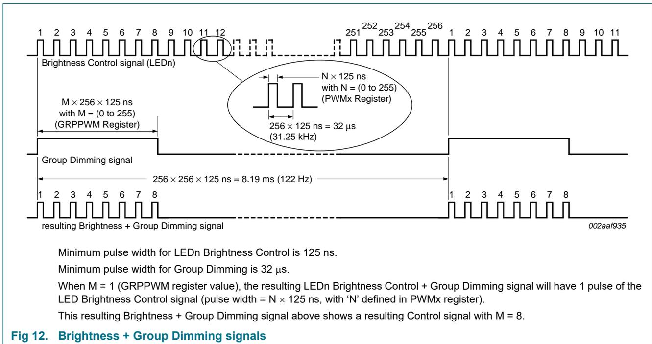
Fig 12. Brightness + Group Dimming signals
