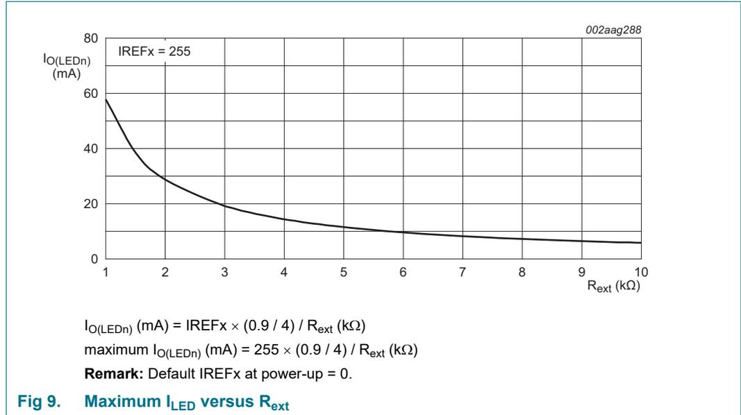
**Example 1:** If  $R_{ext} = 1 \text{ k}\Omega$ ,  $I_{O\_LED\_MIN} = 225 \mu\text{A}$ ,  $I_{O\_LED\_MAX} = 57.375 \text{ mA}$  (as shown in [Figure 10](#)).
