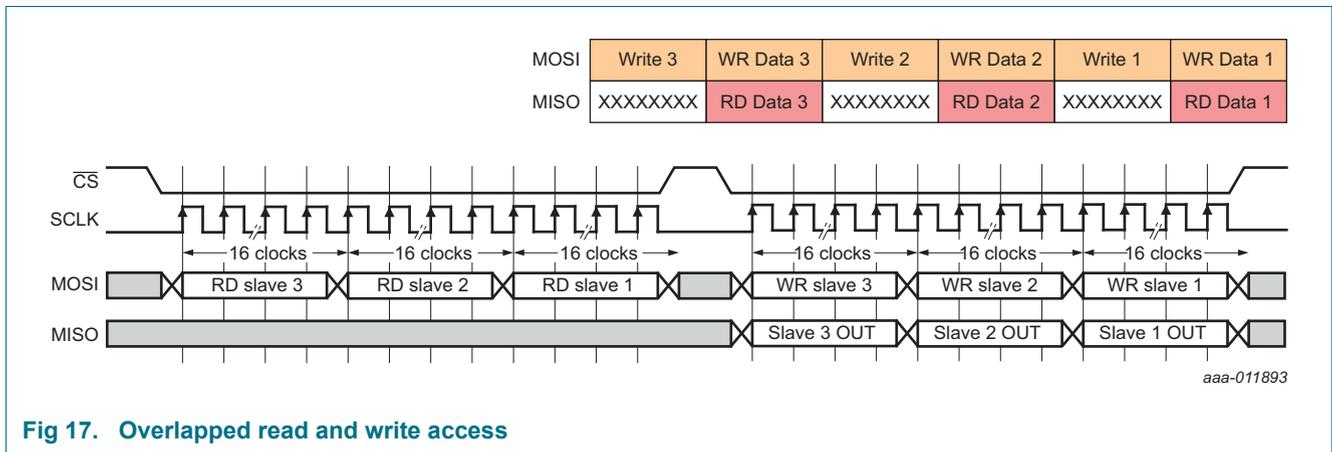
**Fig 17. Overlapped read and write access**
