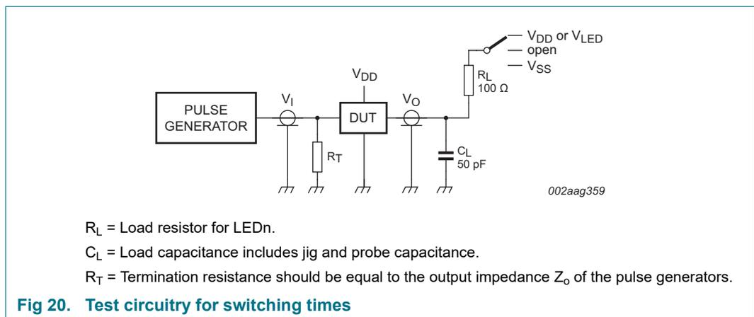
Fig 20. Test circuitry for switching times
