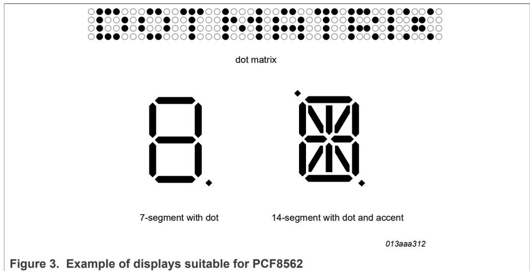
Figure 3. Example of displays suitable for PCF8562
