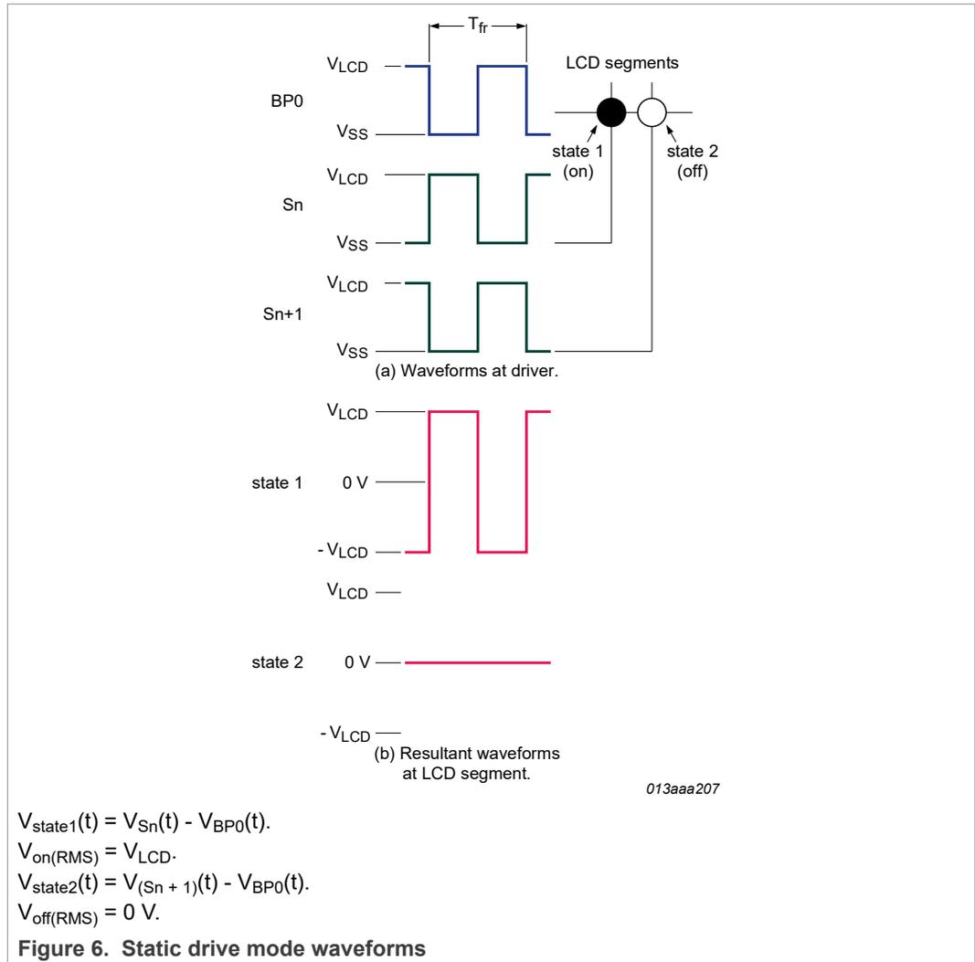
Figure 6. Static drive mode waveforms
