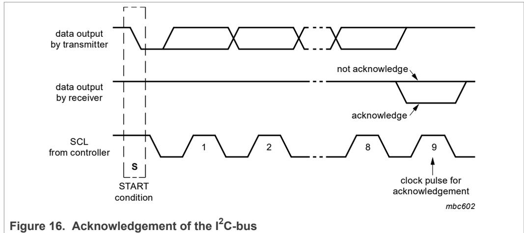
Figure 16. Acknowledgement of the I<sup>2</sup>C-bus
