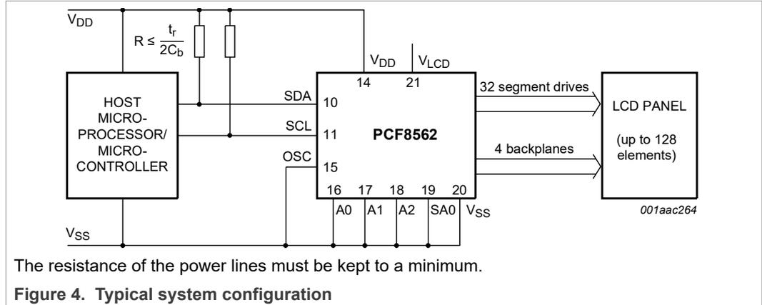
The host microcontroller maintains the 2-line I<sup>2</sup>C-bus communication channel with the PCF8562. The internal oscillator is enabled by connecting pin OSC to pin V<sub>SS</sub>. The appropriate biasing voltages for the multiplexed LCD waveforms are generated internally. The only other connections required to complete the system are to the power supplies (V<sub>DD</sub>, V<sub>SS</sub>, and V<sub>LCD</sub>) and the LCD panel chosen for the application.
