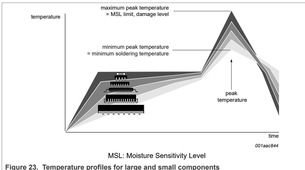
Figure 23. Temperature profiles for large and small components
