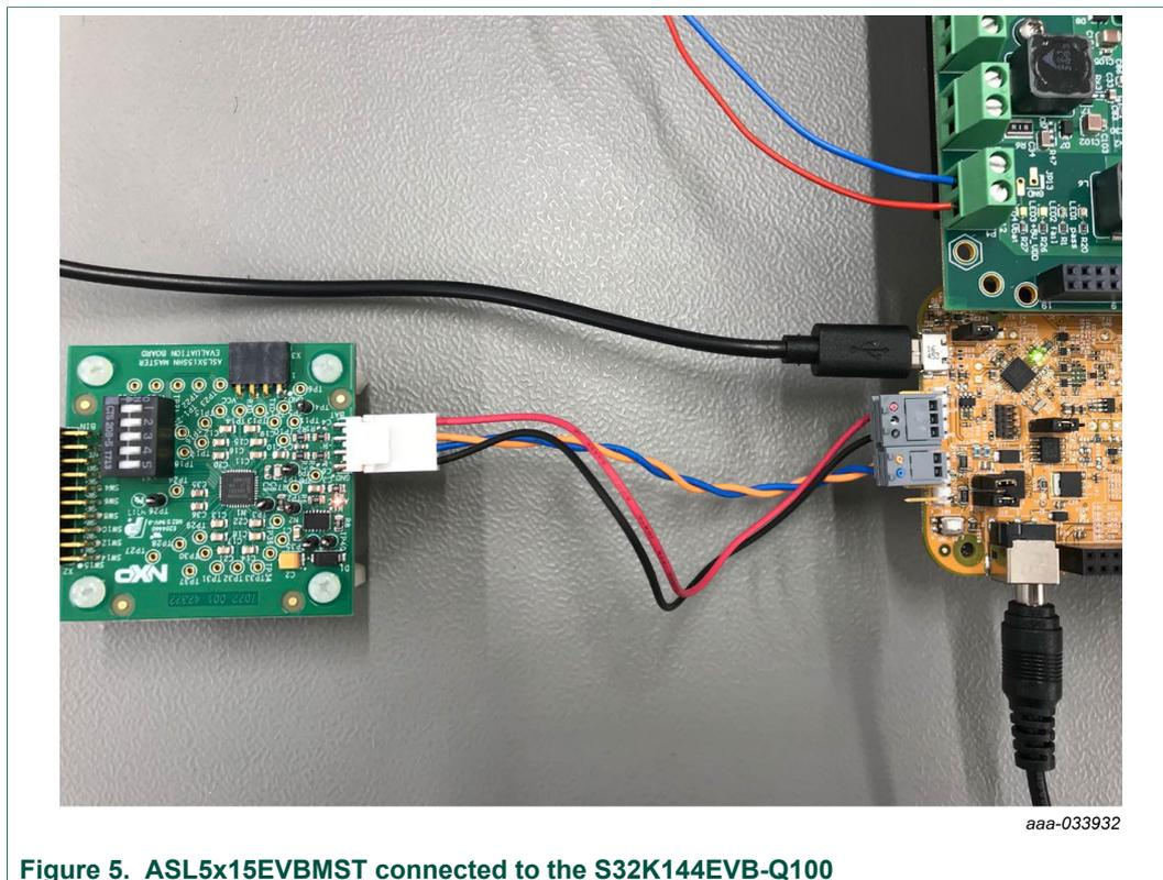
Figure 5. ASL5x15EVBMS1 connected to the S32K144EVB-Q100
