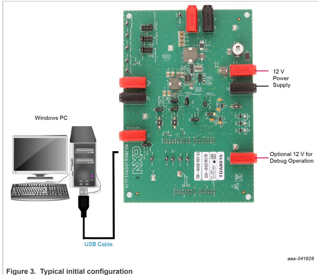
Figure 3. Typical initial configuration
