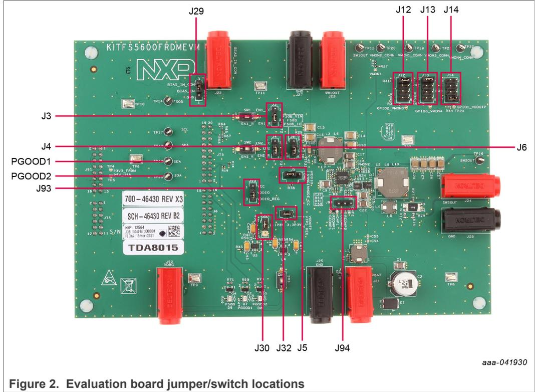
Figure 2. Evaluation board jumper/switch locations
