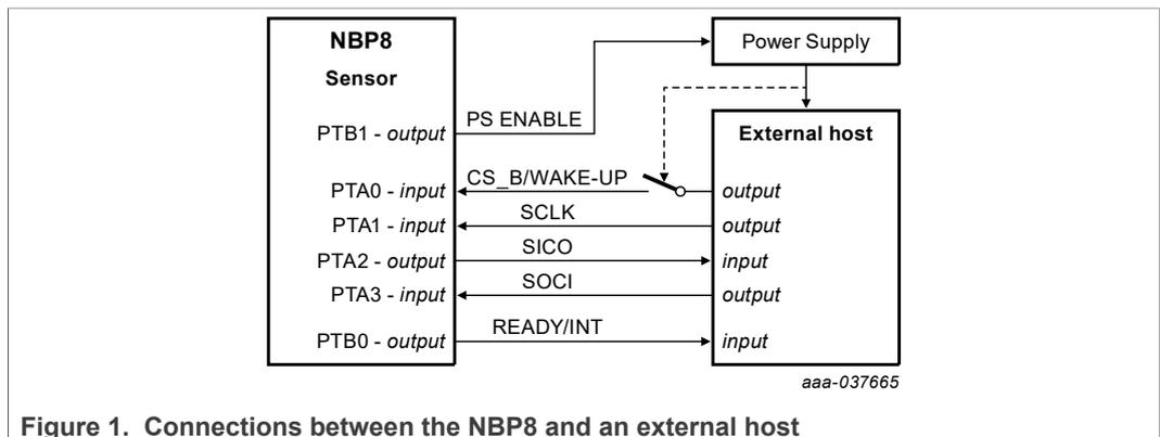
Figure 1. Connections between the NBP8 and an external host
