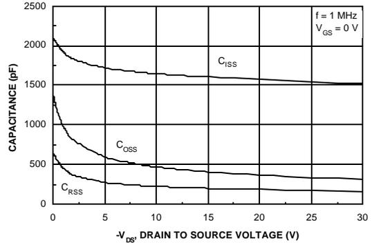
Figure 8. Capacitance Characteristics.
