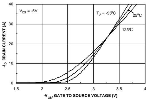
Figure 5. Transfer Characteristics.
