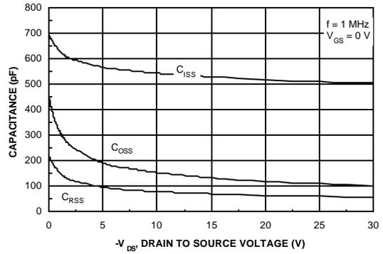
Figure 8. Capacitance Characteristics.
