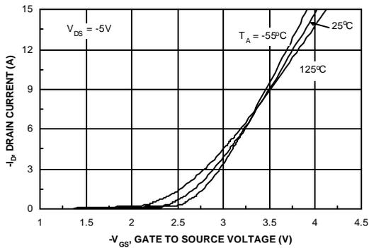
Figure 5. Transfer Characteristics.
