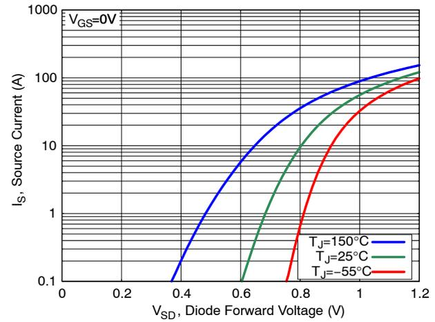
Figure 4. Diode Forward Voltage vs. Source Current
