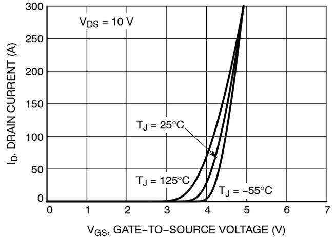
Figure 2. Transfer Characteristics
