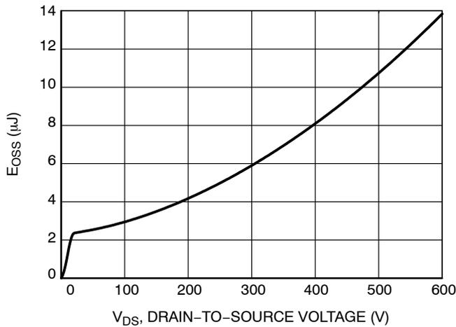
**Figure 11. E<sub>OSS</sub> vs. Drain-to-Source Voltage**
