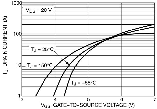
Figure 2. Transfer Characteristics
