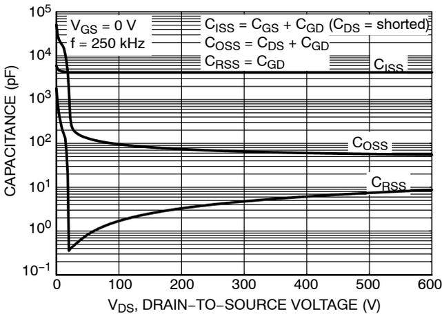
Figure 5. Capacitance Characteristics
