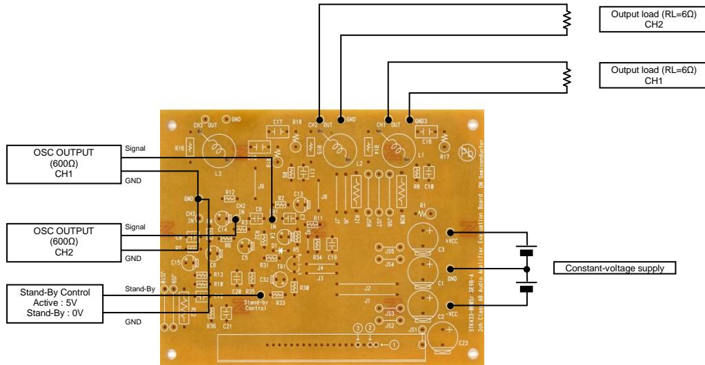
Sound quality confirmation, load short-circuit test, noise examination
