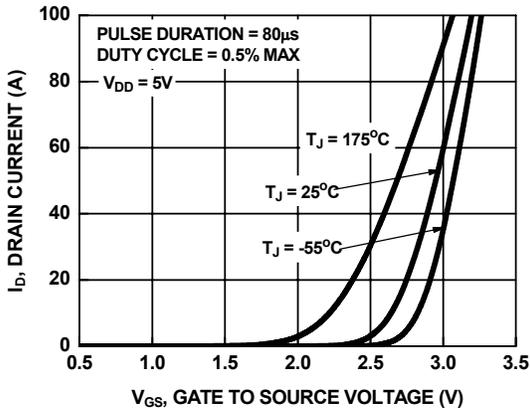
Figure 7. Transfer Characteristics
