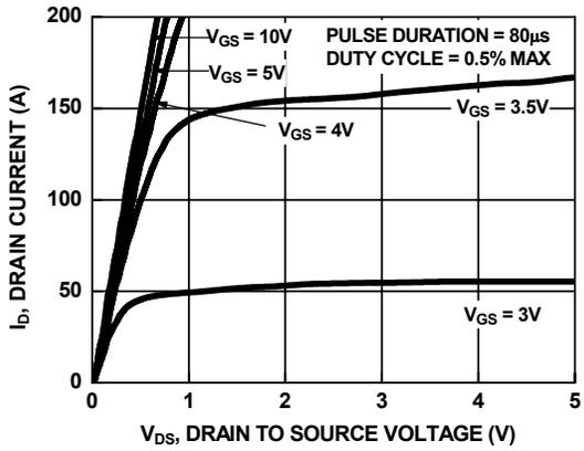
Figure 8. Saturation Characteristics
