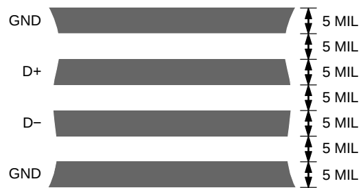
Figure 22. Typical Arrangement of Signal Tracks
