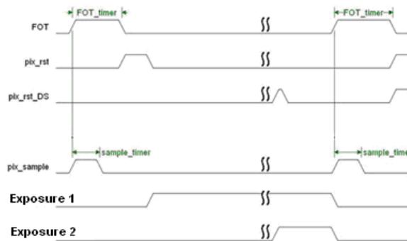
**Figure 37. Dual Slope Timing in Slave Mode**
