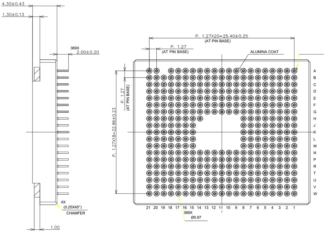
Figure 40. LUPA3000 μPGA Package Diagram (Bottom View)
