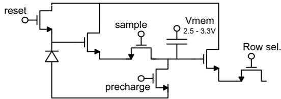
**Figure 8. Pixel Schematic**
