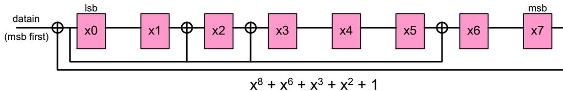
**Figure 11. Equivalent Polynomial Representation in Serial Format**
