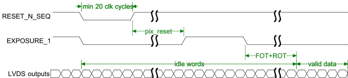
**Figure 34. Sequencer Reset**
