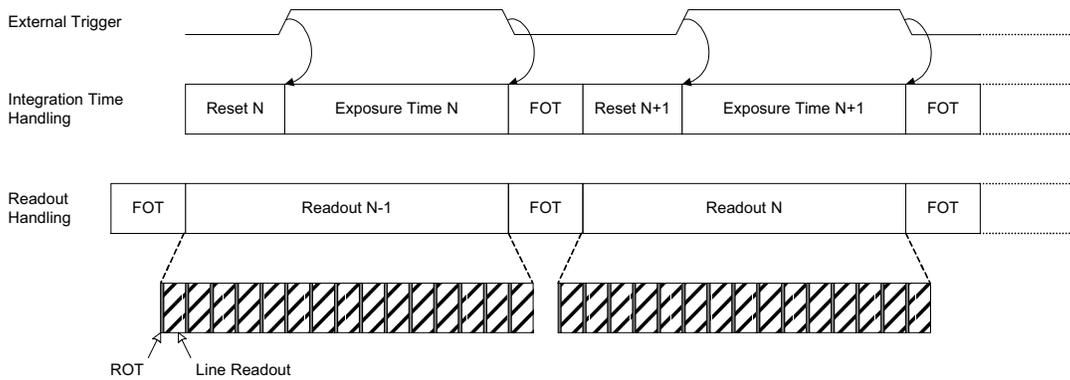
**Figure 20. Pipelined Shutter Operated in Slave Mode**
