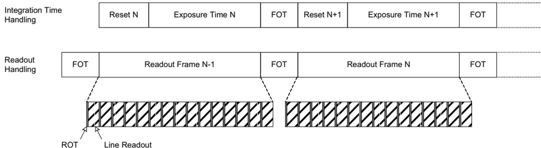
Figure 19. Integration and Readout for Pipelined Shutter
