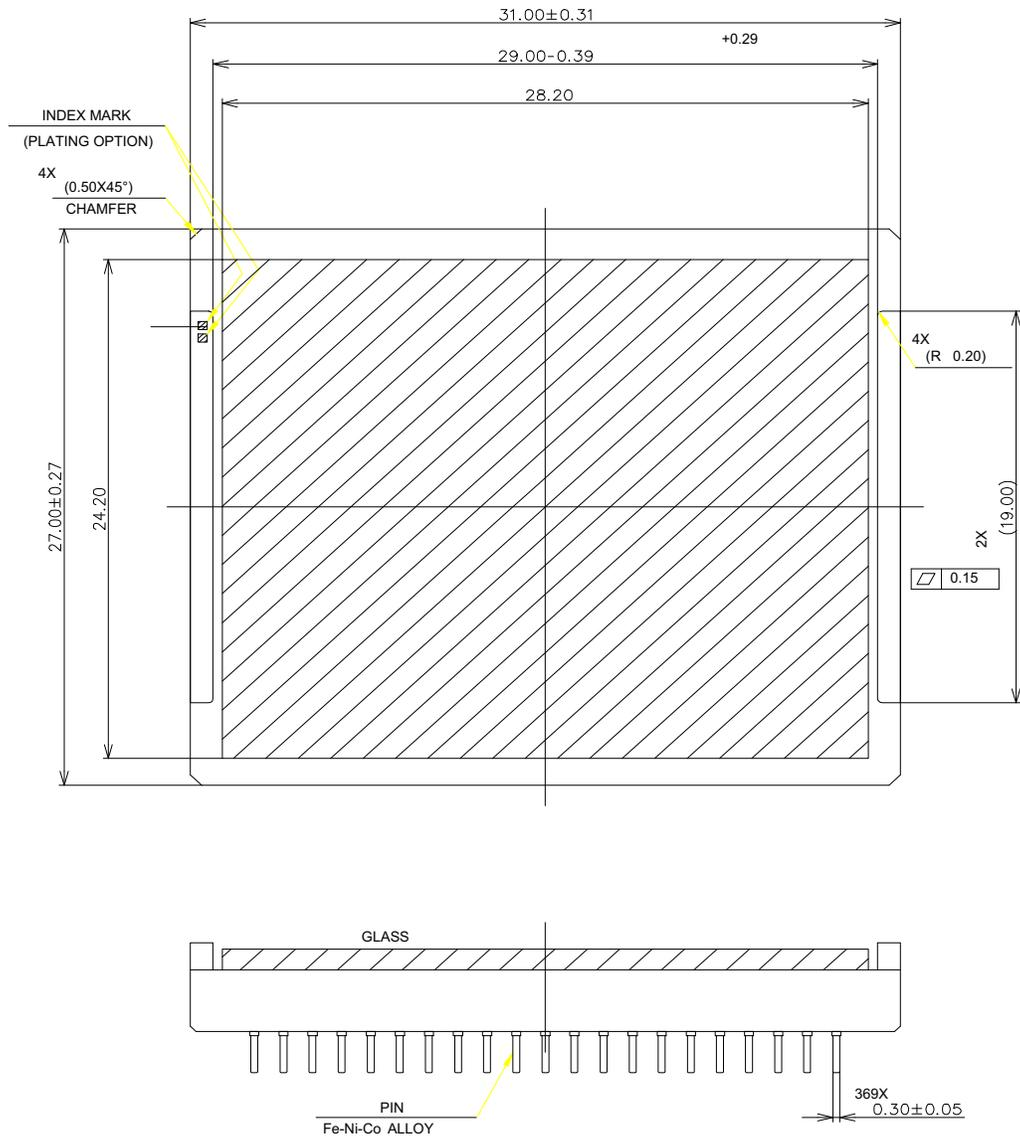
Figure 39. LUPA3000 μPGA Package Diagram (Top View)
