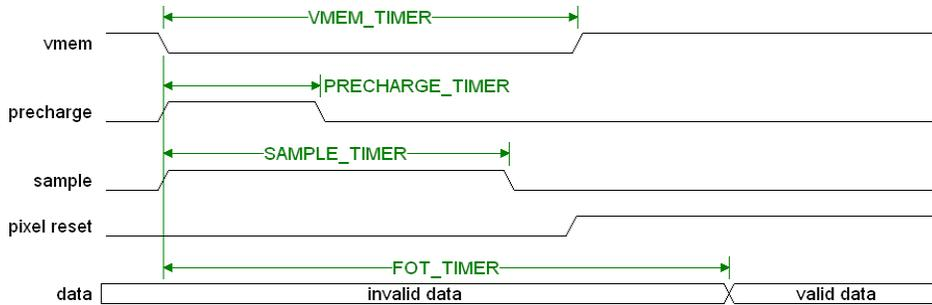
Figure 22. Pixel Timing
