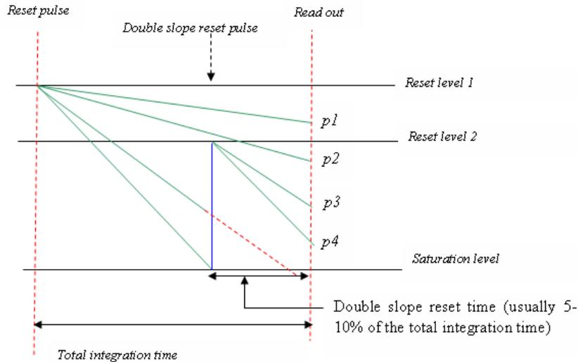
**Figure 36. Dynamic Range Extended by Double Slope Capability**
