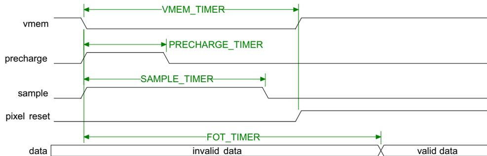
**Figure 30. FOT Timing**
