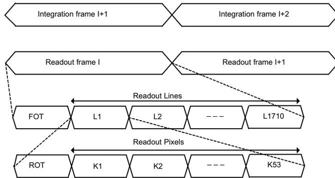
**Figure 25. Pipelined Operation**
