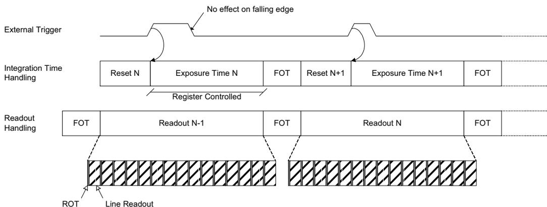
**Figure 21. Triggered Shutter Operated in Master Mode**
