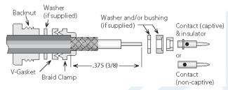
Trim cable jacket to dimension A. Slide backnut, washer, V-gasket, and braid clamp onto cable as shown. Cable jacket should bottom on step in braid clamp.
