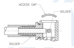
2) Insert prepared cable into rear of body, with all braid wires on outside of crimp tail. Push cable in until the end of braid touches connector body shoulder and center conductor rests in contact slot. Trim excess braid wires even with shoulder of body
