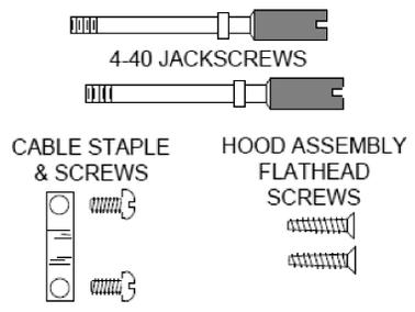
KIT CONSISTS OF TWO MOLDED ABS PLASTIC HALF HOODS, TWO NICKEL PLATED BRASS JACKSCREWS, TWO SELF TAPPING ASSEMBLY SCREWS, AND ONE CABLE STRAIN RELIEF STAPLE WITH TWO SELF TAPPING SCREWS
