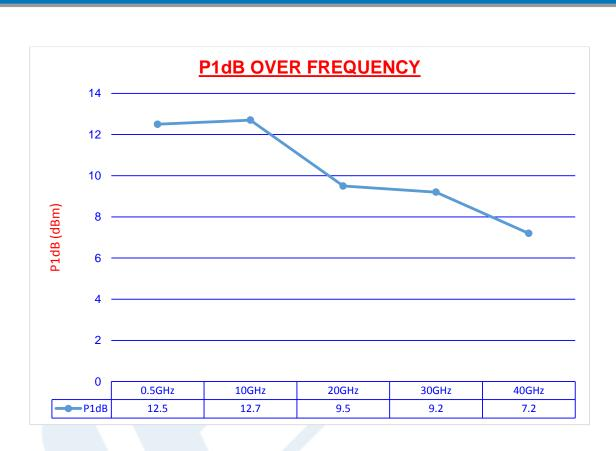
10 dBm P1dB, 50 MHz to 40 GHz, USB Controlled Broadband Amplifier, 12 dB Gain, 2.92mm from Pasternack Enterprises has same day shipment for domestic and International orders. Our RF, microwave and millimeter wave products maintain a 99% availability and are part of the broadest selection in the industry.
