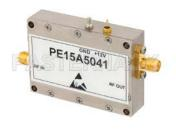
6 Watt P1dB, 800 MHz to 960 MHz, High Power Amplifier, SMA Input, SMA Output, 37 dB Gain, 50 dBm IP3, 3 dB NF
