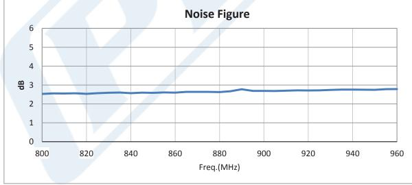
Click the following link (or enter part number in "SEARCH" on website) to obtain additional part information including price, inventory and certifications: 6 Watt P1dB, 800 MHz to 960 MHz, High Power Amplifier, SMA Input, SMA Output, 37 dB Gain, 50 dBm IP3, 3 dB NF PE15A5041
