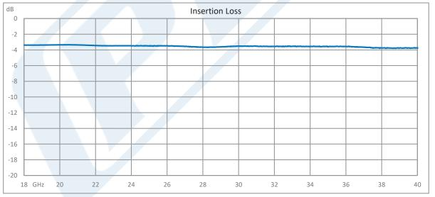
Click the following link (or enter part number in "SEARCH" on website) to obtain additional part information including price, inventory and certifications: 2 Way 2.92mm Power Divider from 18 GHz to 40 GHz Rated at 20 Watts PE20DV1064
