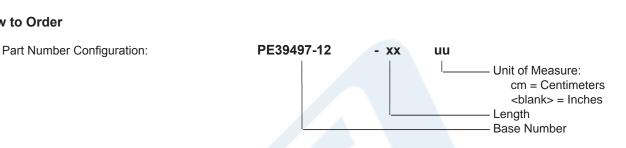
PE39497-12-12 = 12 inches long cable Example: PE39497-12-100cm = 100 cm long cable
