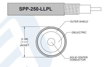
Click the following link (or enter part number in "SEARCH" on website) to obtain additional part information including price, inventory and certifications: Plenum QMA Male to SMA Male Right Angle Low PIM Cable 36 Inch Length Using SPP-250-LLPL Coax , LF Solder PE3C5893-36
