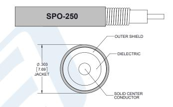
SPO-250 Coax Using Times Microwave Parts PE3C6343-12
