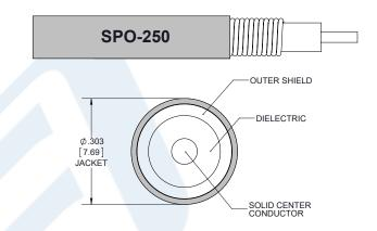
SPO-250 Coax Using Times Microwave Parts PE3C6343-36
