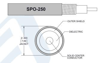
SPO-250 Coax Using Times Microwave Parts PE3C6343-50CM
