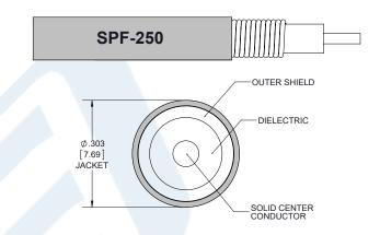
SPF-250 Coax Using Times Microwave Parts PE3C6358-36
