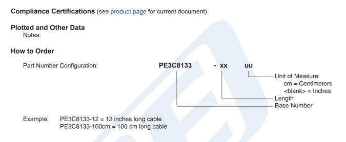
SMA Female to Trimmed Lead Test Probe Cable 12 Inch Length Using PE-SR047FL Coax from Pasternack Enterprises has same day shipment for domestic and International orders. Our RF, microwave and millimeter wave products maintain a 99.4% availability and are part of the broadest selection in the industry.
