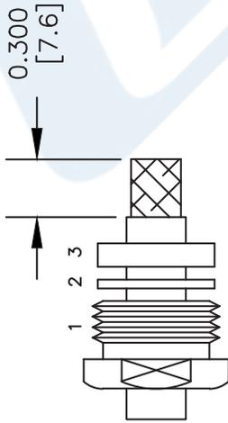
2. FORM BRAID OVER CLAMP NUT (4). TRIM BRAID BACK TO SHOULDER. CUT DIELECTRIC & CENTER CONDUCTOR TO DIMENSION SHOWN. DO NOT NICK CENTER CONDUCTOR. SOLDER CONTACT TO CENTER CONDUCTOR. REMOVE EXCESS SOLDER. DO NOT OVER HEAT DIELECTRIC. INSERT CABLE ASSEMBLY INTO BODY & TIGHTEN.
