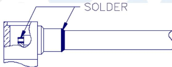
3. SOLDER CENTER CONDUCTOR TO CONTACT.
