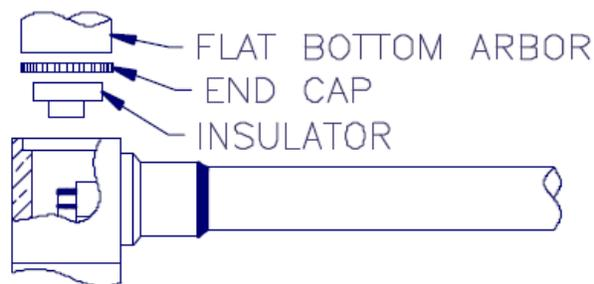
5. PRESS INSULATOR AND END CAP INTO CONNECTOR BODY AND USE A FLAT BOTTOM ARBOR TO PRESS CAP IN PLACE. CAP MUST BE BELOW BODY SURFACE TO SEAT PROPERLY.
