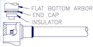
5. PRESS INSULATOR AND END CAP INTO CONNECTOR BODY AND USE A FLAT BOTTOM ARBOR TO PRESS CAP IN PLACE. CAP MUST BE BELOW BODY SURFACE TO SEAT PROPERLY.
