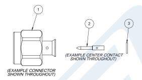
STRIP CABLE AS SHOWN, CHAMFER CENTER CONDUCTOR AND DEBURR CABLE.
