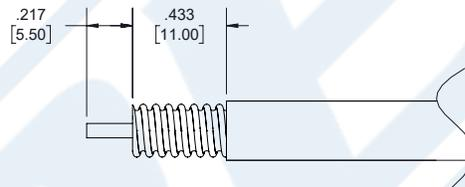
2. SLIDE INSULATOR ③ OVER CABLE CENTER CONDUCTOR. INSERT CENTER CONTACT AND SOLDER. WRAP THE CABLE BY SOLDER WIRE.
