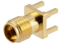
2.92mm Female PCB Mount Connector Solder Attachment Thru Hole, .200 Inches x .059 Inches Hole Spacing 40GHz VSWR1.2
