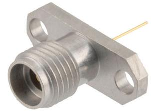
2.92mm Female 2 hole PCB Mount with Round Contact 42GHz VSWR1.2, 0.012 Inches Diameter Pin and 0.315 Inches Pin Length
