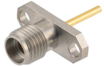
2.92mm Female 2 hole PCB Mount with Round Contact 42GHz VSWR1.2, 0.050 Inches Diameter Pin and 0.413 Inches Pin Length
