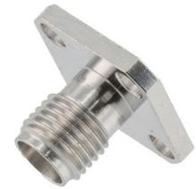
2.92mm Female 4 hole 0.5 inches SQ with Round Contact 40GHz VSWR1.2, 0.012 Inches Diameter Pin and 0.059 Inches Pin Length
