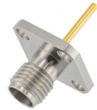
2.92mm Female 4 hole SQ 0.5 Inches with Round Contact 42Ghz VSWR1.2, 0.050 Inches Diameter Pin and 0.413 Inches Pin Length
