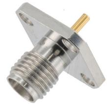
2.92mm Female 4 hole SQ 0.5 Inches with Round Contact 40GHz VSWR1.2, 0.050 Inches Diameter Pin and 0.197 Inches Pin Length
