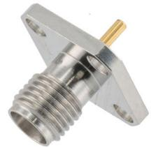
2.92mm Female 4 hole SQ 0.5 Inches with Round Contact 40GHz VSWR1.2, 0.050 Inches Diameter Pin and 0.197 Inches Pin Length
