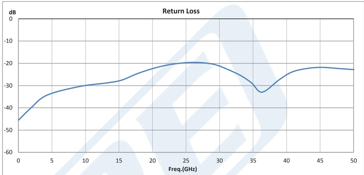
1 Watt RF Load Up to 65 GHz With 1.85mm Male Input Passivated Stainless Steel from Pasternack Enterprises has same day shipment for domestic and International orders. Our RF, microwave and millimeter wave products maintain a 99% availability and are part of the broadest selection in the industry.
