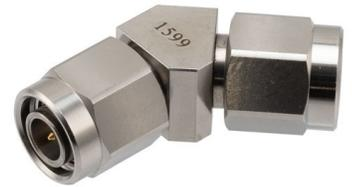
RF Adapter, 45 Degree Angle TNC plug to TNC plug 18GHz VSWR1.2
