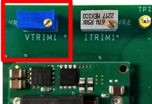
The user can change the output voltage through the trim potentiometer. VTRIM1(VR1) is for PS1, VTRIM2(VR101) is for PS100.
