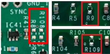
The two i7C modules must be synchronized to a common switching frequency during parallel operation. This function is enabled as default setting and the required clock signal (refer to i7C product specification) is provided on the evaluation board to synchronize the module’s switching at approximately 250KHz. To disable the sync during independent operation (not required), remove R8 and R108 and install R9 and R109.
