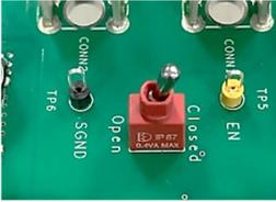
Changing position of toggle switch SW1 to “Closed” turns-on both PS1 (Master) and PS100 (Slave) DC-DC modules. By default, SW1 is connected to the ON/OFF pins of both PS1 and PS100 modules through R1 and R101 (See schematic for more details).
