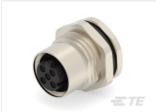
TE Part #T4131512041-000 M12,REAR MOUNT,FEMALE,D,4P, SOLDER WIRE
