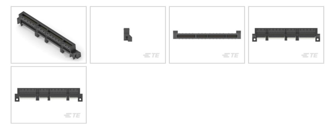
Internal I/O Connector Type: Sliver for SFF-TA-1002 Connector Mates With: PCB Edge Card PCB Mount Orientation: Straddle Mount Number of Positions: 168 Industry Standard: Gen-Z, OCP NIC 3.0
